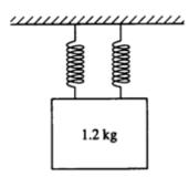
Two identical massless springs are hung from a horizontal support. A block of mass 1.2 kilograms is suspended from the pair of springs, as shown above. When the block is in equilibrium, each spring is stretched an additional 0.15 meter.
