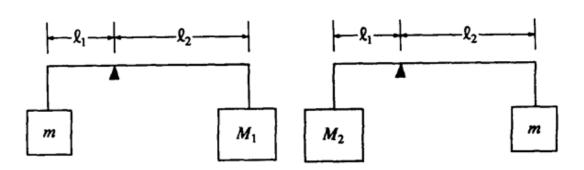
35. A rod of negligible mass is pivoted at a point that is off-center, so that length l<sub>1</sub> is different from length l<sub>2</sub>. The figures above show two cases in which masses are suspended from the ends of the rod. In each case the unknown mass m is balanced by a known mass, M<sub>1</sub> or M<sub>2</sub>, so that the rod remains horizontal. What is the value of m in terms of the known masses?
